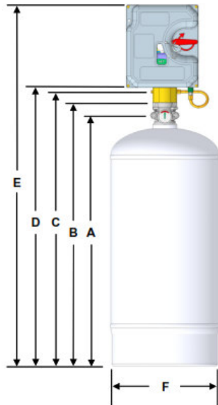
Figure 2. Dimensions of Cylinder Assembly with SVA and XV Control System
