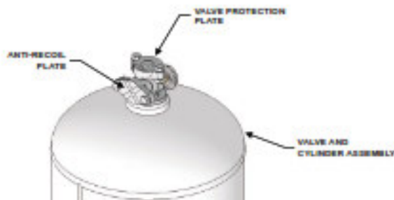
Figure 4. Anti-Recoil and Valve Protection Plates
